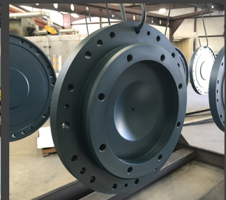
Interlock Piston Rod Socket Coated w/ Xylan 1052 #595 100%
