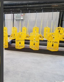
Subsea Labels Coated w/ 4 Coat Subsea System
