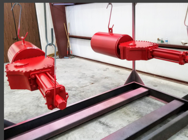
Actuators/Gearbox Coated w/ 3 Coat system (red) 2 Coat system (grey)
